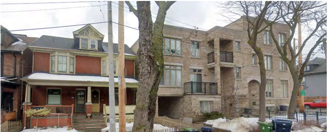
Figure 54: The multi-unit infill building (right) maintains the street character through similar setback to the the existing homes. Taller elements of the infill building are located at the corner, and parking is located behind the building.
