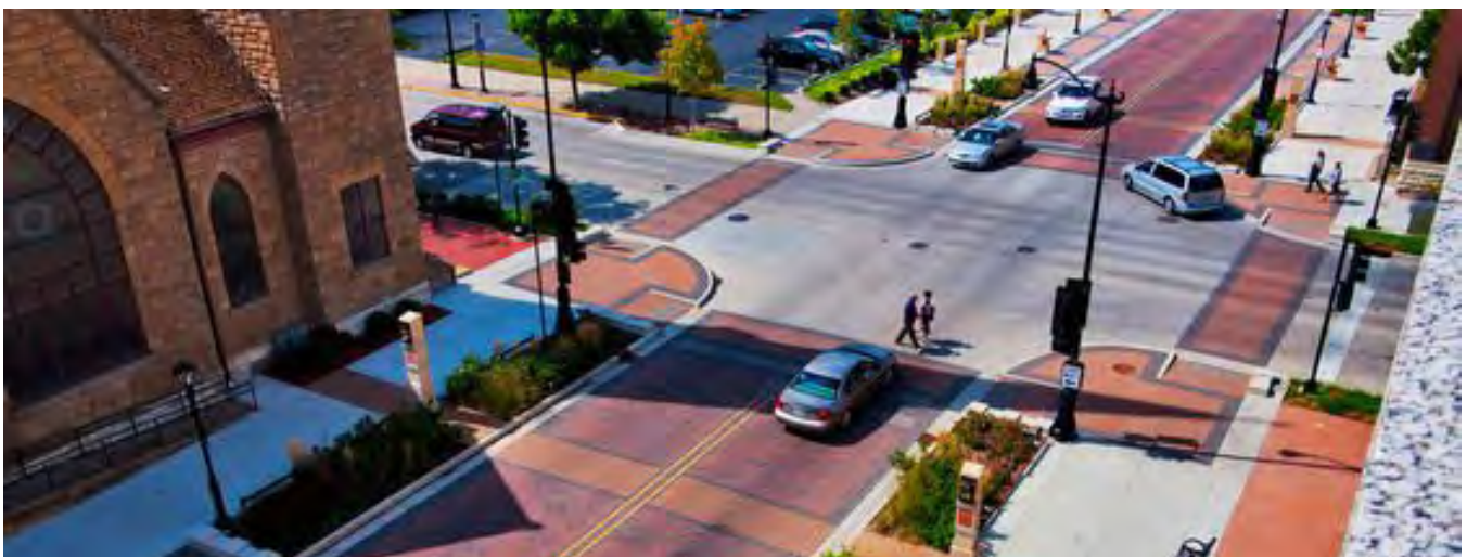
Figure 30: Shared street designs provide pedestrian-oriented streetscaping elements across the entire right-of-way, from building face to building face. While accommodating vehicles and/or parking, the shared street design prioritizes active transportation. It can be closed to vehicular traffic during events or seasonally, providing a flexible urban plaza for gathering and activities.
